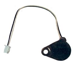
Mounts under ISN-SM Series Seismic Detectors, directly on the mounting plate or on the supervised surface. The mechanical oscillations from the test transmitter are propagated in the surface as vibrations. The seismic detector picks up the vibration signals and triggers an alarm if the detector is functioning correctly. This tests not only the detector itself, but also the physical contact between the detector and the protected object.
