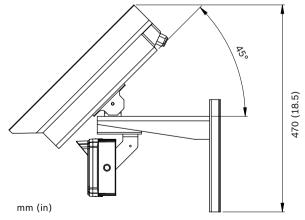
Camera housing tilted to maximum elevation.
